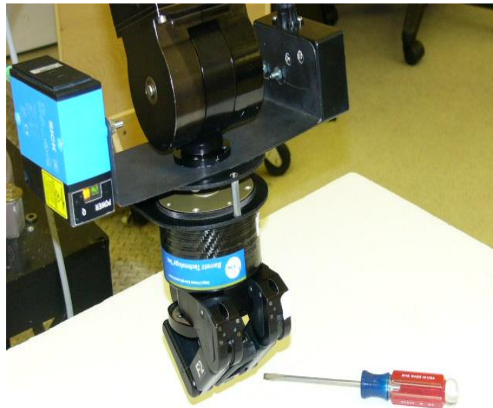
Figure 7.4 Camera and the Sick DT60 Laser Range Finder Mounted at the Puma's End-Effector
